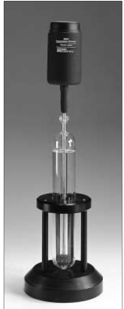
Hart's new Model 2031 Immersion Freezer "Quick Stick" makes the formation of ice mantles in triple point of water cells easy. Just fill the reservoir with dry ice and alcohol (or liquid nitrogen) and come back in an hour to find a thick, evenly formed ice mantle. No baby-sitting required.
